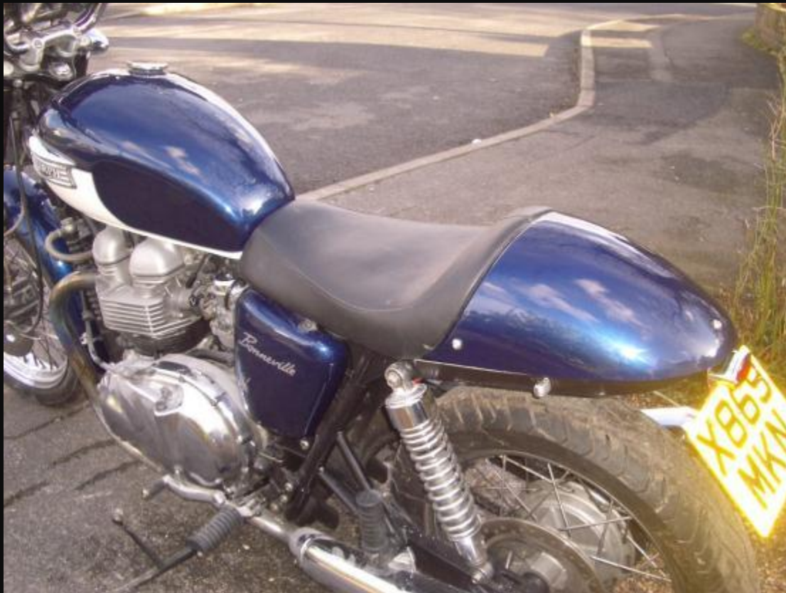
Solo Seat and eliminator fitted to an early 2001 Bonneville.
