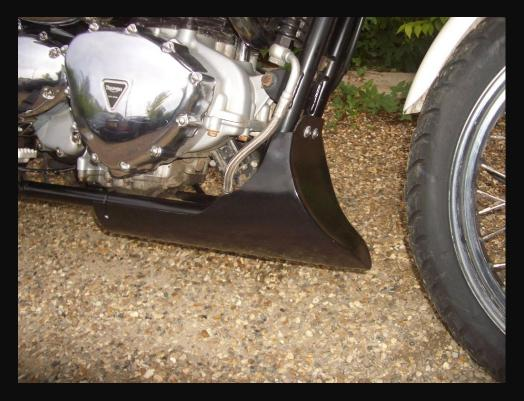
If you look at the belly pan in black unpainted GRP you will see how it fits. The front is held on with two stainless bolts and spacers that fit into the existing plate fitted on the front of the down tubes. The back is held on with two cable ties. Ten minute job to fit and very quick to remove when you need to change the oil.
