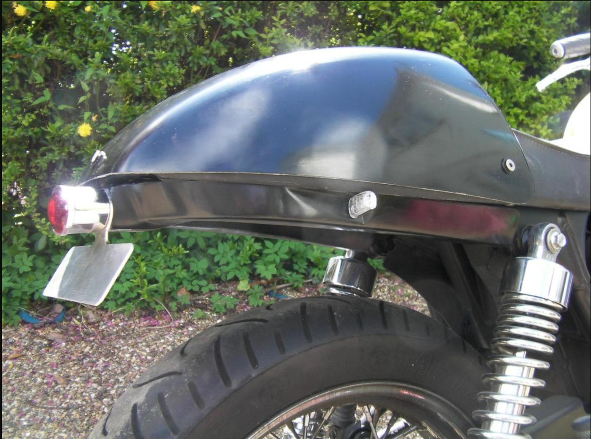
This is the finished result, you will need to have the cowl painted, temporary screws are fitted here, stainless button screws are supplied.
