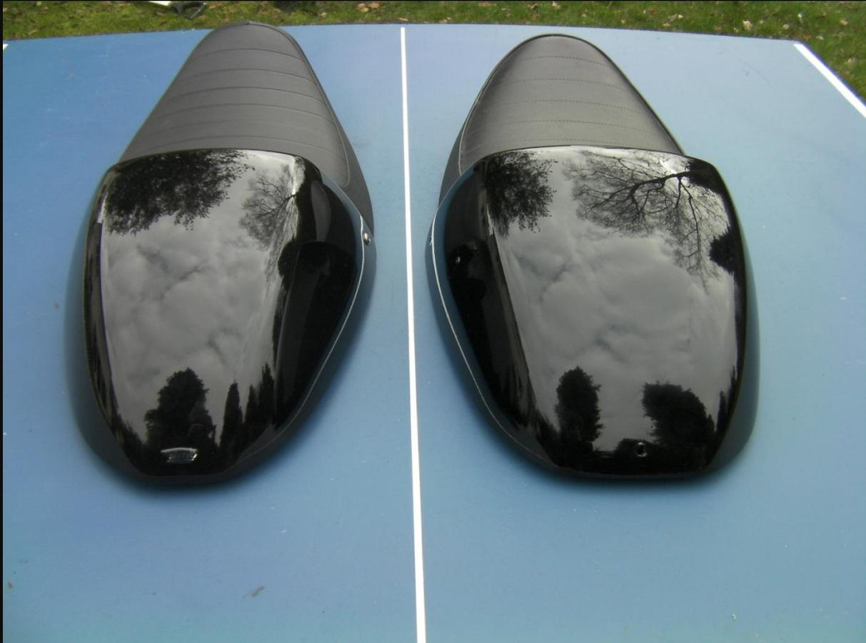
The cowl on the left is the standard cowl as fitted to the original Triumph Thruxton, the one on the right is my modified cowl designed to fit the standard Bonneville seat. You can clearly see from the pictures that it is quite a bit wider than the Thruxton version.
