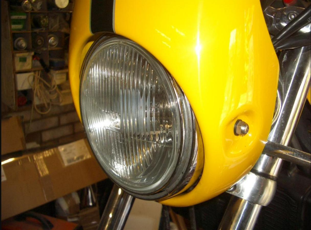
Fit the bolt and washer to the other side, inserting a Philips screwdriver first helps to align the hole.
